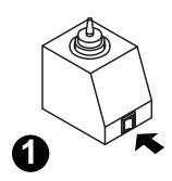
Facing the front of the unit, find the red power switch in the lower, center or the unit. Turn the power to the OFF position. The light will go out.
