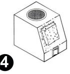
Wash\* inside and outside with a sponge, cloth or cleaning pad using a mild soap solution. For "hard water" spots and scale, scrub the area\*\* using a strong solution of vinegar and water. Let stand for 5 minutes.
