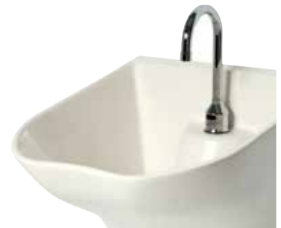
Thin outside rim is angled downward to discourage users from placing objects on it, reducing infection.
