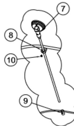
Figure 2: Installing thermometer
